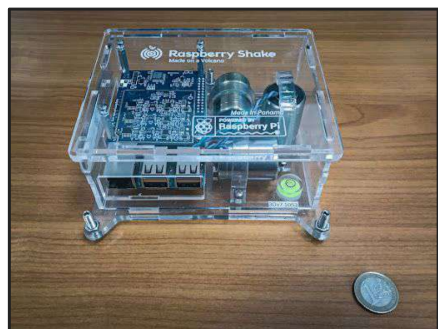
Figure 1: Example of a Raspberry Shake seismic station (3D model) used in the project.
